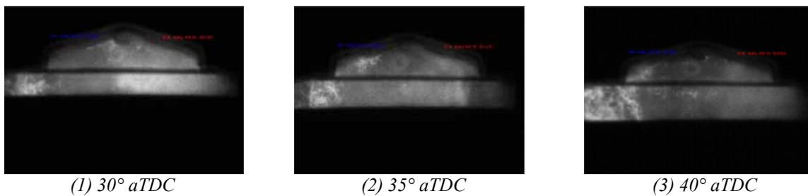
*Fig. 7. Occurrence of single flames (surface ignition) – sequence of flame images (side view)
