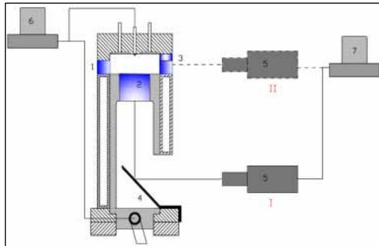
Fig. 2. Experimental apparatus for combustion test – two optical paths used to carry out experiment
