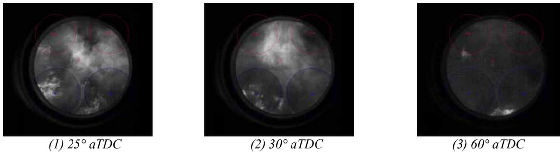
*Fig. 6. Occurrence of single flames (surface ignition) – sequence of flame images (bottom view)
