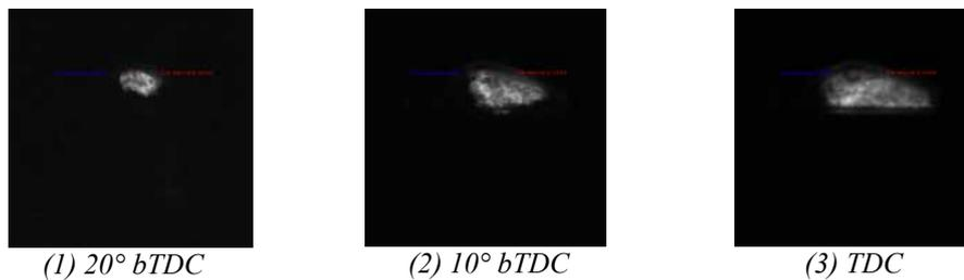
Fig. 4. Spark-ignition combustion process – sequence of flame images (side view)
