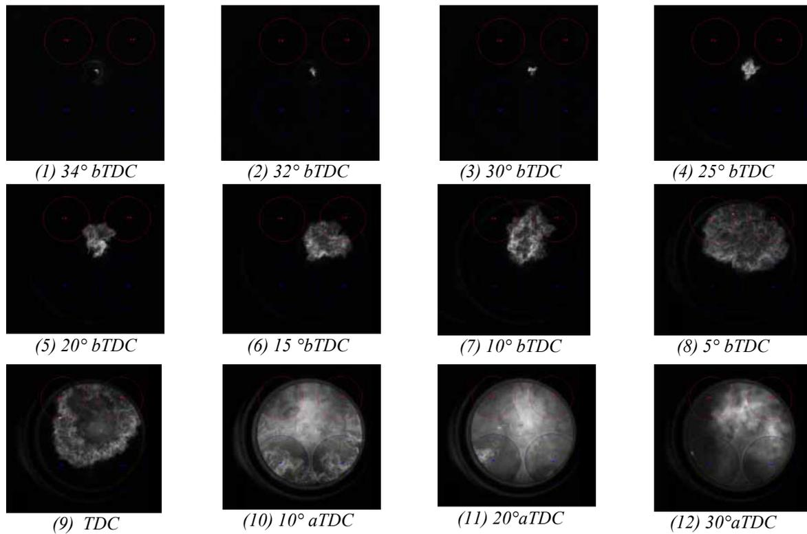
Fig. 3. Spark-ignition combustion process – sequence of flame images (bottom view)
